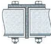
CAPTIVE INSTALLATION BETWEEN ALUMINUM H-BEAMS ACOUSTIBLOK PART # 2ALUMIBEAM
