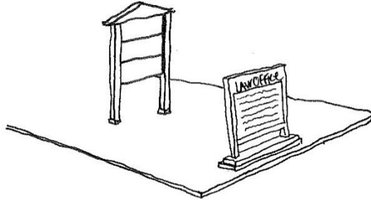
Ladder Sign and Ground Sign
