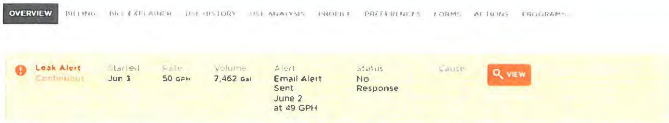
Figure 4: Customer Portal Leak Alert. Image of VXengage portal (previously known as the WaterSmart portal) provided by VertexOne, care of Scotts Valley Water District.
