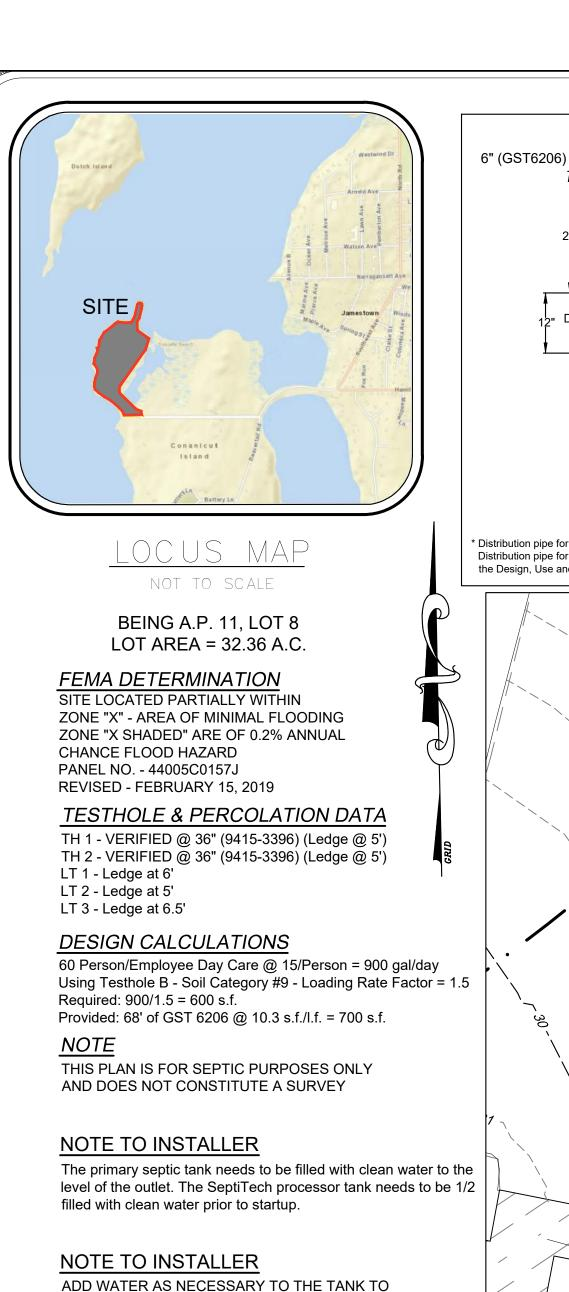
ADD WATER AS NECESSARY TO THE TANK TO COUNTERACT ANY BUOYANT FORCES ACTING UPON THE STABILITY OF THE TANK POSITION WHEN INSTALLING A
