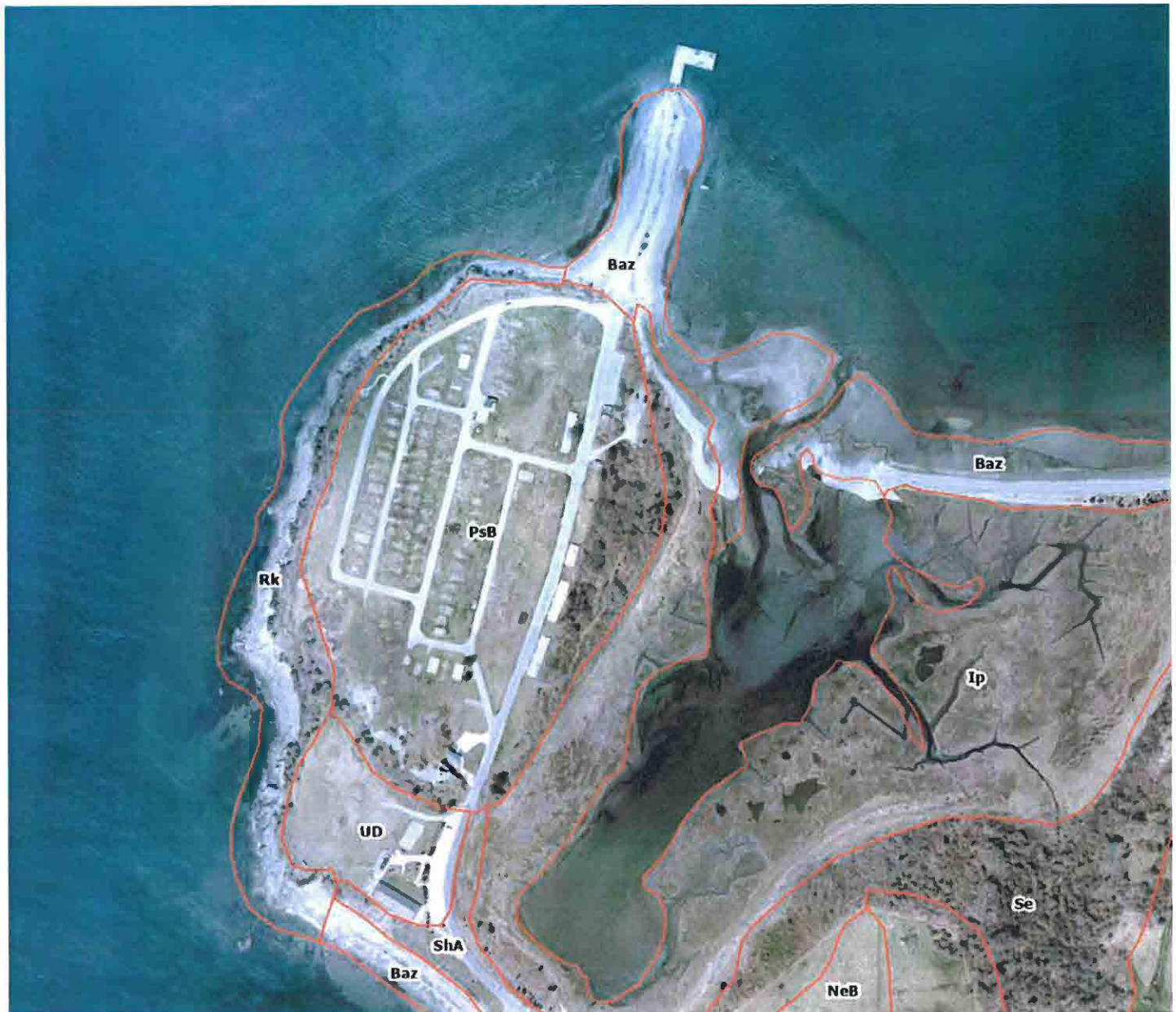
Figure 3. Soil Mapping Units in the Vicinity of Fort Getty, Jamestown, Rhode Island
