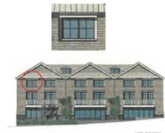
Sill is recessed and head is emphasized. No "picture-framed" on four sides.
