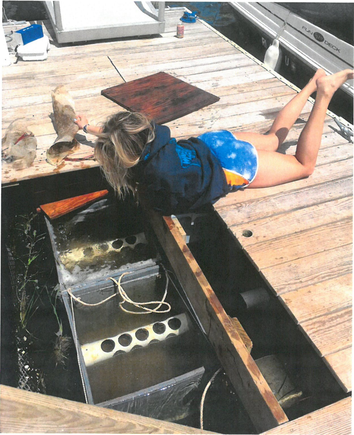
Photo 2. Current upweller in Ninigret Pond with trap doors open to access juvenile oysters in silos.
