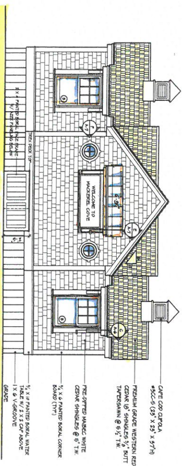
3 FRONT ELEVATION SCALE: 1/4" = 1'-0"
