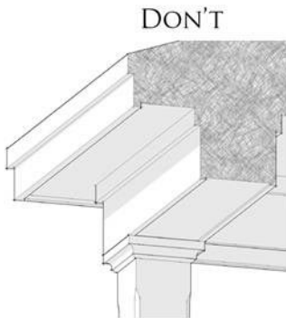
25.2 Avoid column capitals that are as wide as the beam. Column capitals should extend beyond the face of the beam. In traditional wood construction, the trim for the capital is applied to the column shaft, which is aligned with the face of the beam.
