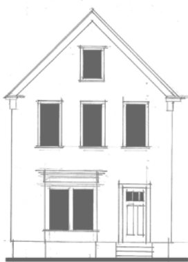
9.2 Attention should be paid to the percentage of solid to void. Enough wall should remain to suggest strength and enclosure.
