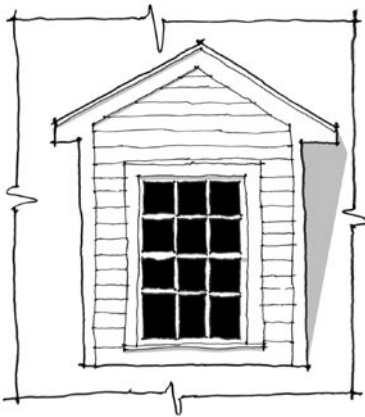
28.4 Avoid detailing dormers such that the window is set within a "wall" and siding is required between the casings and the corner.
