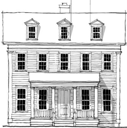
27.1 Dormer placement is based on the window pattern below, but does not repeat it. The distance between eaves is at least twice the width of the window.
