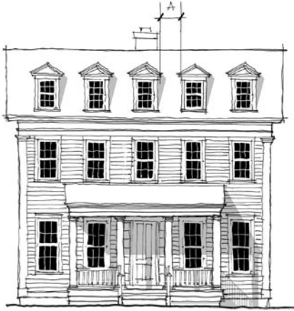
28.1 Avoid spacing dormers too closely with uncomfortably tight clearance at the eaves.
