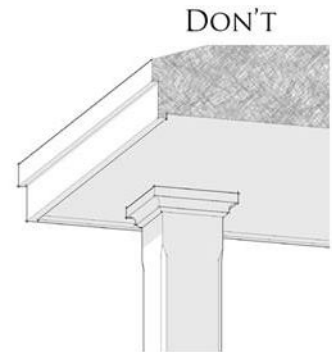
25.4 Avoid details that eliminate the use of a beam altogether. Columns that support the ceiling directly appear ready to puncture the ceiling surface. Beams are meant to support the roof and should not be omitted from the assembly.
