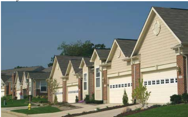
4.2 Locating the garage doors in the same plane as the principal structure creates a very uninviting presence. The garages and homes become indistinguishable from one another.
