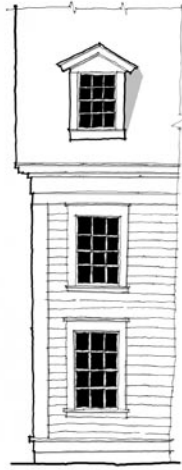
28.2 A smaller window means the entire dormer looks proportional to the main windows.
