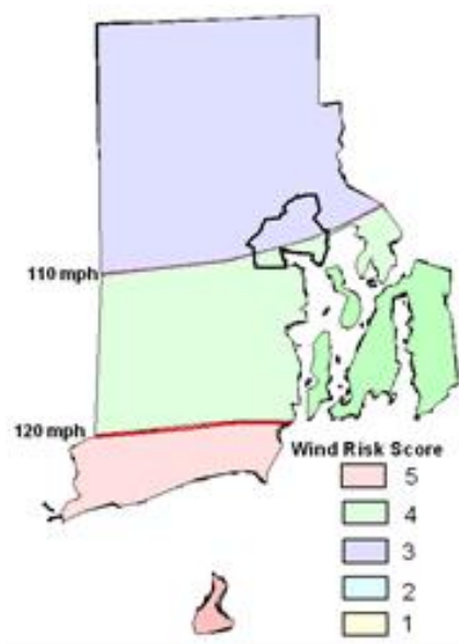
Figure 3-2. Wind risk score for Rhode Island Source: American Society of Civil Engineers
